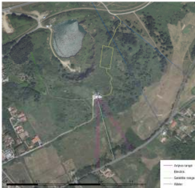
Figure 4. The utilities within the Alderney Community Woodland site. The exact site of the electric cable within the yellow box is unknown, but will be located following further clearance work.
